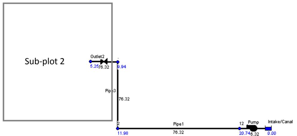
The system delivers to the sub-plot 2 a Flow rate of 76.32 m<sup>3</sup>/hour with a Pressure of 5.25 m.w.c and a flow velocity of 1.24 m/s (figure 7).
